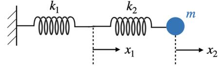
$$\begin{aligned} -k_1x_1 + k_2(x_2 - x_1) &= 0 \\ \Leftrightarrow x_1 &= \frac{k_2}{k_1 + k_2}x_2 \end{aligned}$$
